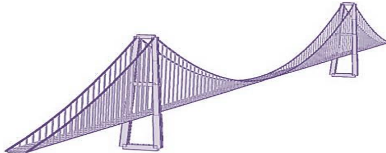
Fig.11: Finite element model of The Great Belt Bridge.
